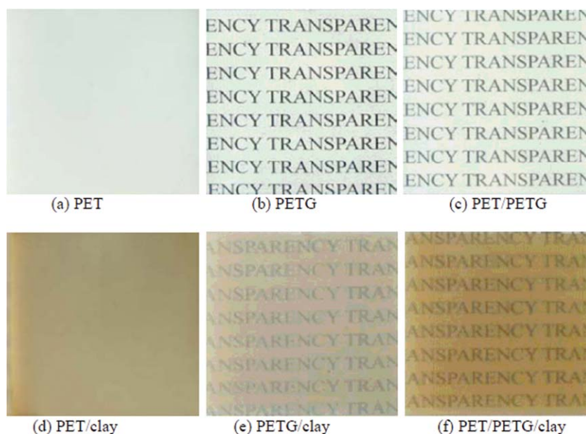
Figure 8. Transparency effects on PET blended with PETG and clay (2 mm thick). [Color figure can be viewed in the online issue, which is available at wileyonlinelibrary.com .]
